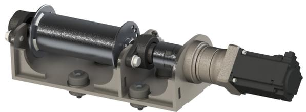
*Initial design of the load generating subsystem prototype*
